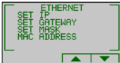
Figure 7-2. Ethernet Communication Setup
