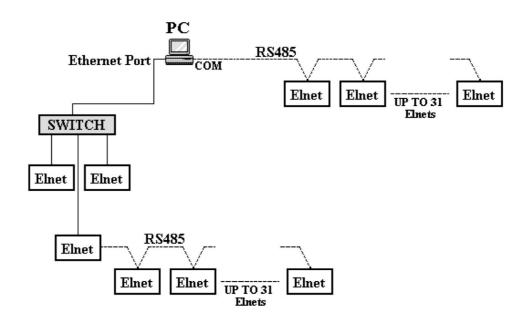
TCP\IP ETHERNET (Shielded & Grounded)
